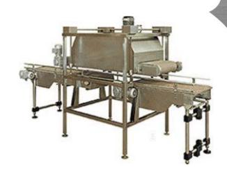
THE SISMATICO VACUUM TRANSFER UNIT CONSISTS OF 3 MODULES; INFEED CONVEYOR - VACUUM TRANSFER - OUTFEED TRANSFER CONVEYOR. THESE 3 UNITS RUN AT A SPEED WHICH IS 12% FASTER THAN THE CAN SUPPLY SPEED WHICH CREATES A NATURAL GAP BETWEEN THE CANS. THIS PREVENTS FALLEN CANS BEING CARRIED INTO THE MASS AIR CONVEYOR SYSTEM.
