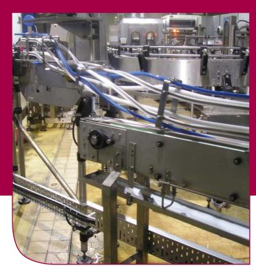
OUR EQUIPMENT IS GENERALLY SUPPLIED WITH MANUAL VENTED TOP COVERS IN 1.25 METER LENGTHS AS STANDARD. THESE CAN ALSO BE SUPPLIED WITH AUTOMATIC MULTI HEIGHT SELECTION SYSTEM AS AN OPTION. THE CAN HEIGHT SELECTION IS MADE FROM THE MAIN CONTROL PANEL.
